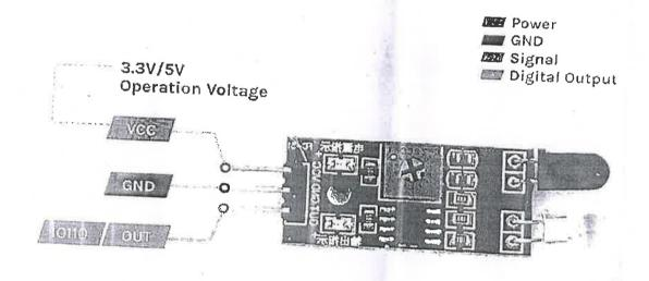
is the power supply pin for the IR sensor which we connect to the 5V pin on the Arduino.
